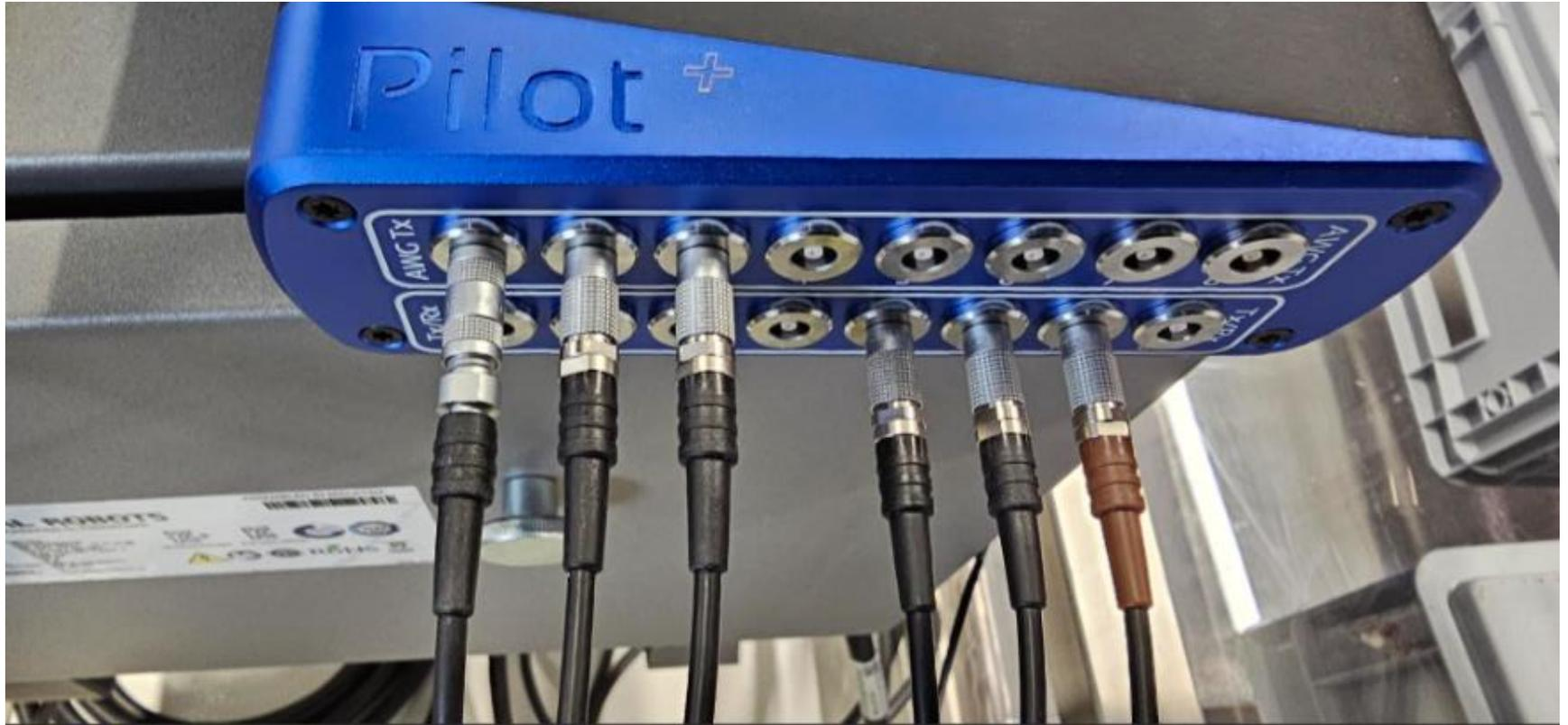
Pilot+ : 8 parallel channel allowing to speed up the inspection
